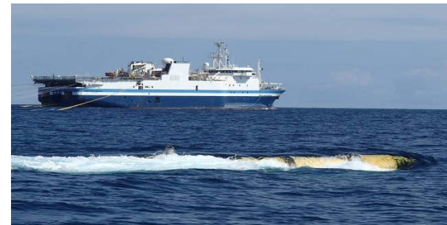
3D Vessel CGG Amadeus – 8 x 8,100m sentinel solid streamers Broadseis and Broadsource (Broadband) Technology
